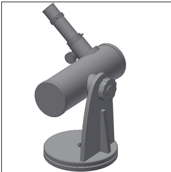
Figure 6. Erecting eyepiece for terrestrial view.
